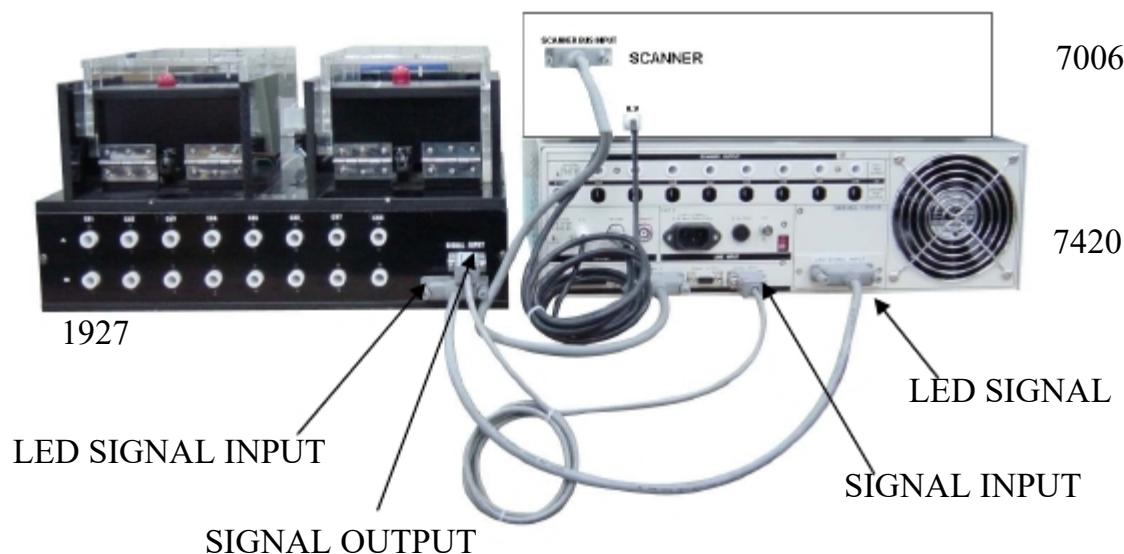
(一) Signal input 9 Pin D-type (MODEL 7420 at Rear panel SIGNAL INPUT socket)
